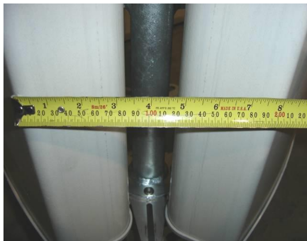
Figure 4.6.1 Measure the distance between outer radii of adjacent antennas
