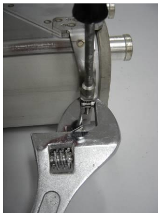
Figure 4.1.4 : A shifter can be used to prevent twisting of the strap when tensioning
