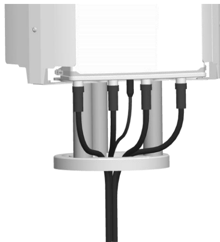
Figure 4.7.1 Cabling of one sector showing four signal cables and one AISG cable
