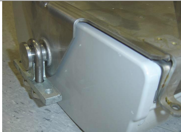
Figure 4.1.2 : The head of the guide pin sits in the cut out of the 'U' Bolt bracket
