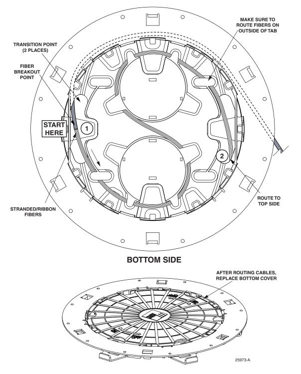
2. Flip the tray over and continue routing cable(s) "A" around the spools and back to the top side, as shown in Figure 5. After routing cable(s) on bottom side, replace bottom cover.
