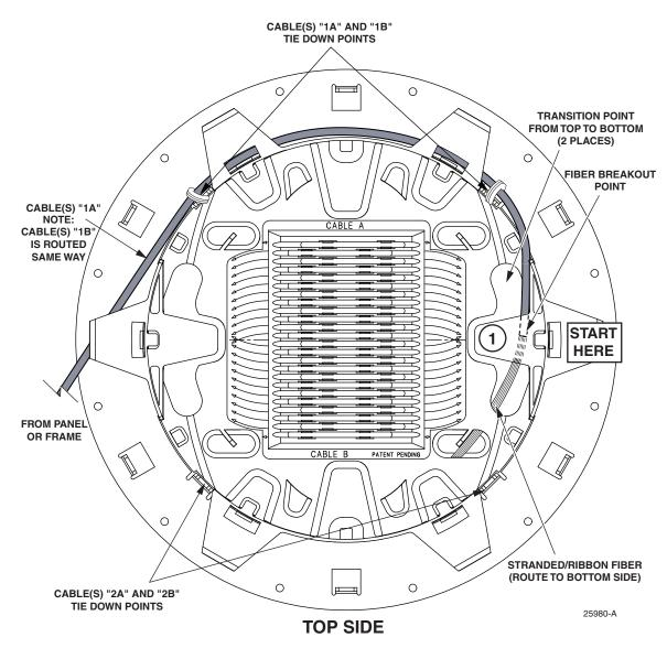
Figure 13. Cable "1A" Routing, Top Side (Clockwise Roll-Up Procedure)
