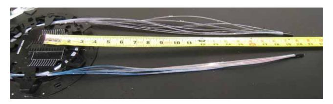
Figure 28. Measuring Pliable Fibers for Cutting
