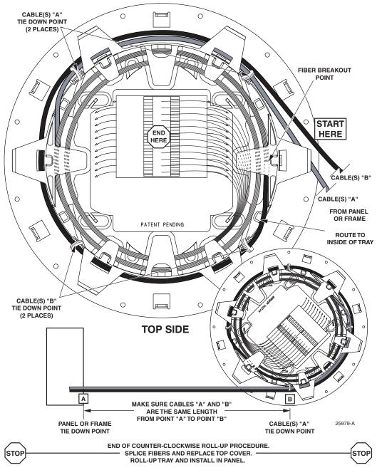
Figure 11. Cable(s) "B" Routing (Counter-Clockwise Roll-Up Procedure)
