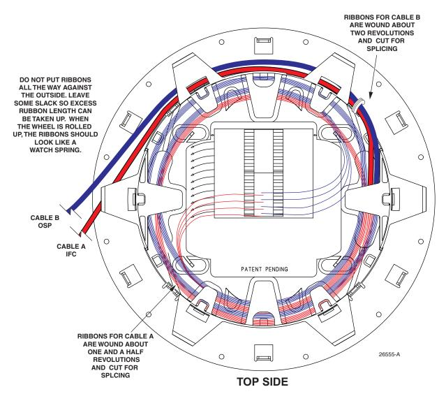
Figure 22. Clockwise Roll-up (4 Stacked Ribbons per Oval Tube)
