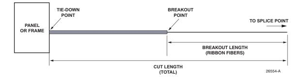
Figure 21. Fiber Ribbon Lengths
