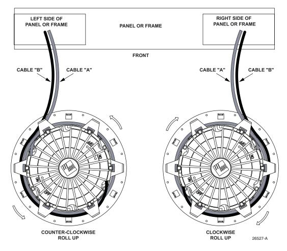
Figure 1. Counter-Clockwise and Clockwise Roll-Up Directions
