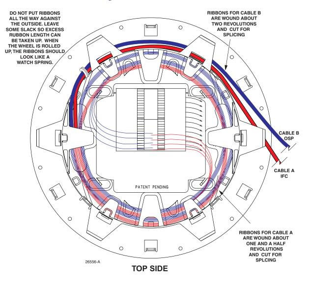
Figure 23. Counter-Clockwise Roll-up (4 Stacked Ribbons per Oval Tube)
