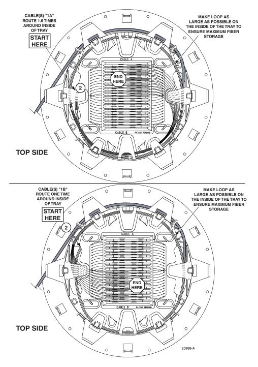
Figure 15. Cable(s) "1A" (Upper View) and Cable(s) "1B" (Lower View) Clockwise Roll-Up Procedure, continued
