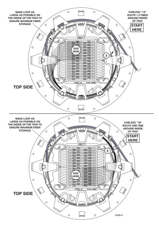
Figure 19. Cable(s) "1A" (Upper View) and Cable(s) "1B" (Lower View) Counter-Clockwise Roll-Up, continued
