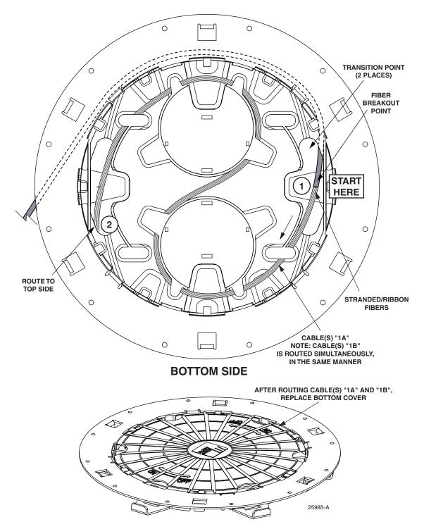
Figure 18. Cable(s) "1A" Routing, Bottom Side (Counter-Clockwise Roll-Up Procedure), continued
