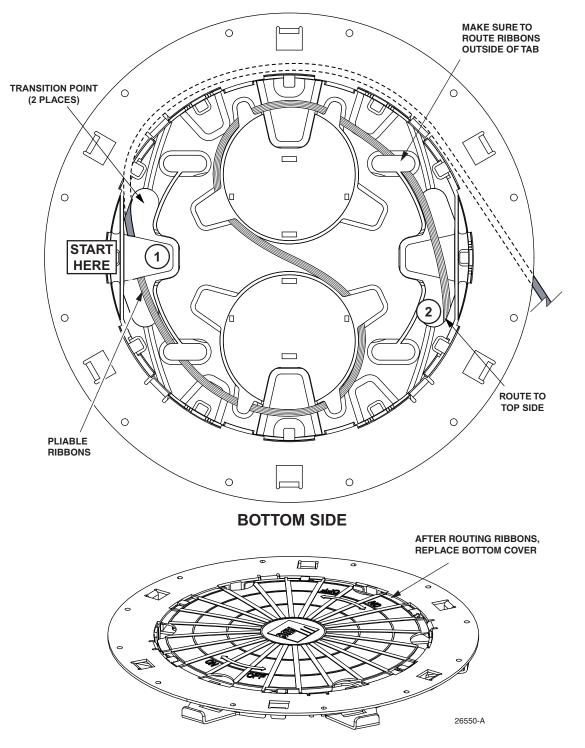
2. Flip the tray over and continue routing the pliable fibers around the spools and back to the top side, as shown in Figure 27. After routing on bottom side, replace bottom cover.
