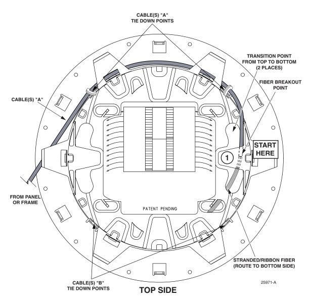
Figure 4. Cable(s) "A" Routing, Top Side (Clockwise Roll-Up Procedure)
