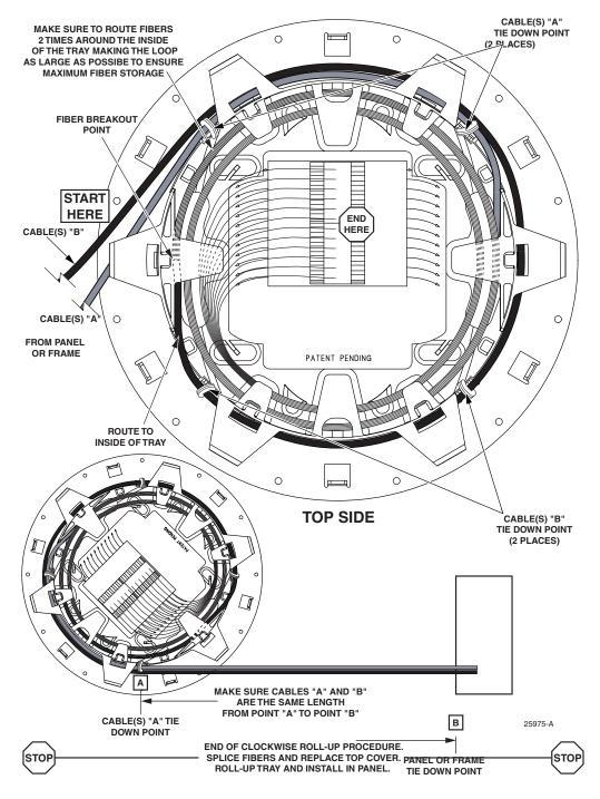
Figure 7. Cable(s) "B" Routing (Clockwise Roll-Up Procedure)
