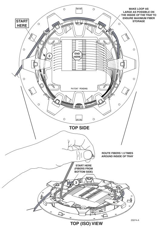
Figure 6. Cable(s) "A" Routing, Top Side (Clockwise Roll-Up Procedure), continued
