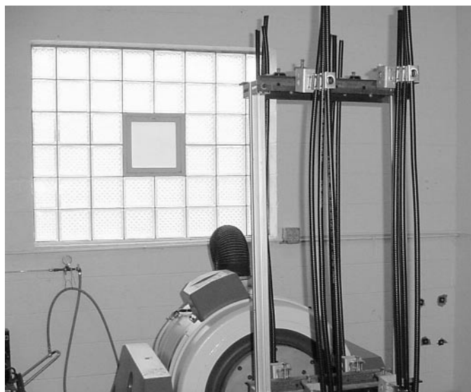
Vibration setup in Y plane. Hangers in 3-out configuration
