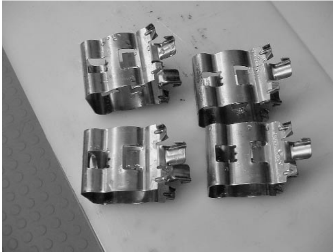
Results - L4 SnapStak™ Hangers after Corrosion Test. No effect
