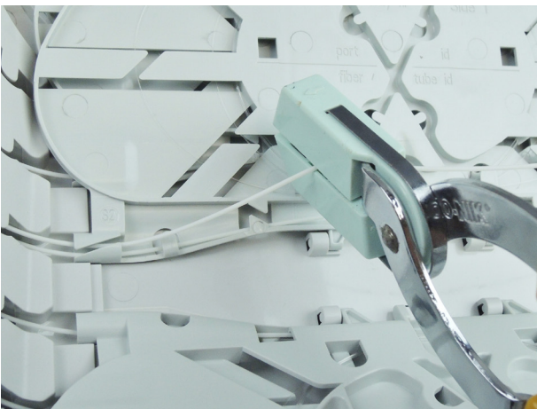
3.6 Strip the 900 \mu m to 250 \mu m with a proper tool
