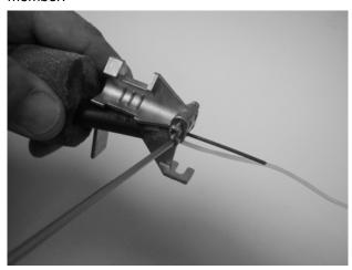
3.6 Cut away the excess of the strength member to make the strength member flush with the cable bracket.
