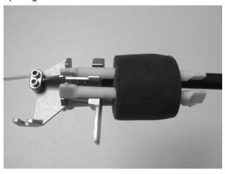
3.9 Install the hose clamp and secure the cable(s) and the cable plug(s) to the bracket.
