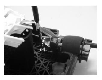
4.3 Secure the cable(s) and cable plug(s) to the closure with the black tie wrap as shown below.
