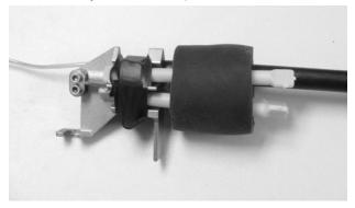
3.11 Select the appropriate blocking ring according to the cable outer diameter. Cut the selected rings on the mark.
