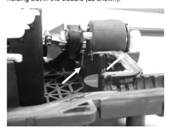
4.2 Secure the cable bracket in the closure with the screw.
