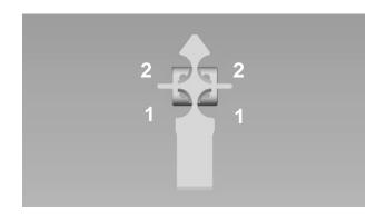
3.4 Install the strength member into its securing cavity and then push the cable to its end position as shown in image below.
