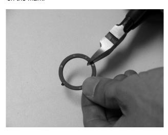
3.12 Install the blocking ring over the cable(s) and the cable plug(s).
