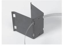
2. Insert the 2 longest metal straps through the slots in the back of the mounting bracket. Fix mounting bracket onto the pole by closing the metal straps around the pole. Fasten the straps with a screwdriver.
