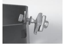
6. Fix the 2 wire clamps onto the mounting bracket. Tighten the nuts off the clamps onto the bracket. Make sure that the clamps are positioned so that the wire is in line with the closure.
