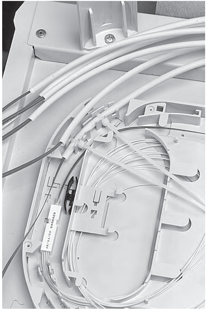
5.4.1 Fix the tubes in the middle position with tie-wraps. Don't squeeze the tubes.
