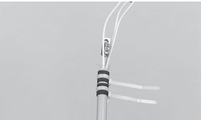
4.2.8 Place the foam and push the tie-wraps onto the cable as shown and install the strength member connector.
