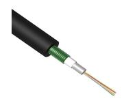
Fiber OSP cable, HDPE, 8-fiber, Singlemode, loose tube, gel-filled, Singlemode G.652.D and G.657.Al, Meters jacket marking, Black jacket color, 1000 m. Provides Rodent Resistance
