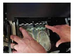
Carefully route fibers as directed in the EHD Chassis Quick Start and User Manual (available using QR code on page 1). Reinstall drawer blade when done.
