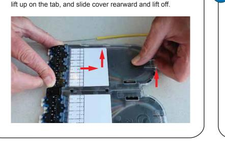
To remove the cover, place a thumb on CommScope icon,
