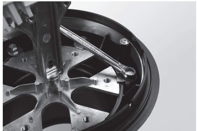
3.1.3 Loosen the securing screws of the cable attachment plate and take out the cable attachment plate with the pre-installed UMS.
