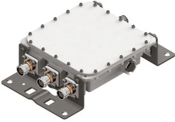
Triplexer 1710-1880/1920-2170/2300-2690, dc bypass on all ports, with 4.3-10 connectors
