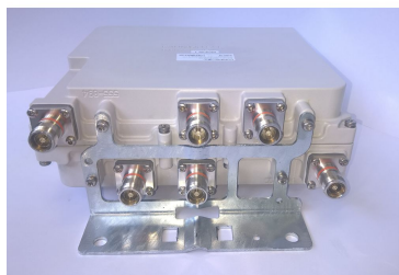
Twin TMA PCS/WCS with 555-894 MHz bypass, 4.3-10 connectors
