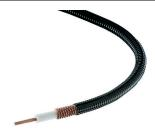
RSJ4-50, HELIAX® Superflexible Foam Coaxial Cable, corrugated copper, 1/2 in, black non-halogenated, fire retardant polyolefin jacket B2ca-sla,d1,a1
