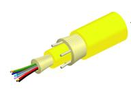
Fiber indoor cable, TeraSPEED® Low Smoke Zero Halogen Riser MPO Trunk, 16-fiber, 3.0 mm subunits, Singlemode G.657.A2/B2, Feet jacket marking, Yellow jacket color, B2ca flame rating
