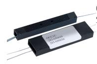
OCC1P Wideband Splitter, planar, singlemode, 1x8, symmetrical split ratio, SC/UPC, 0.9 mm cable, medium duty housing
