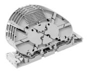
FIST® Splice Sub-assembly kit with 5 trays, each for holding up to 12 primary or 4 secondary coated fibers, with Heat Shrink type splice holder
