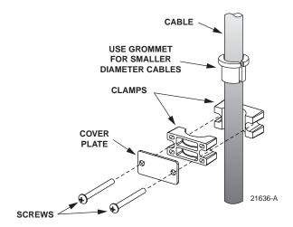
Figure 21. Cable Clamp Assembly
