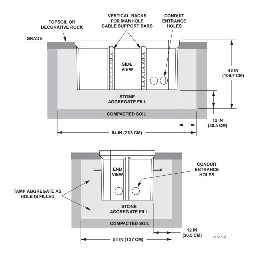
Figure 4. Excavation Recommendations for FMS-ACE100-KIT-A
