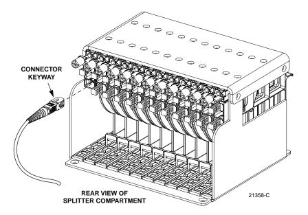
Figure 18. Feeder Cable Connector
