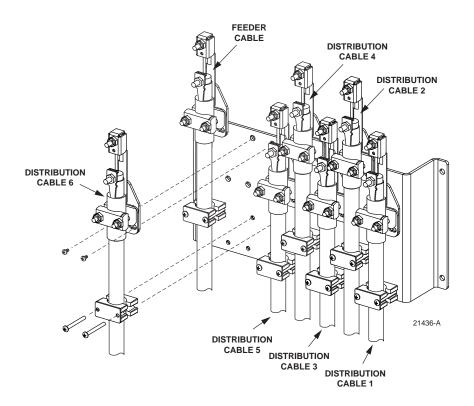
Figure 20. Secure Distribution Cable to Cable Bracket
