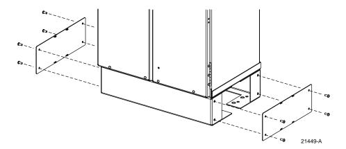
Figure 13. Removing Side Access Covers From Ground Spacer/Riser
