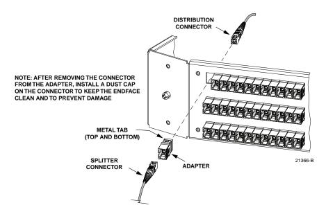
Figure 35. Adapter Removal and Replacement
