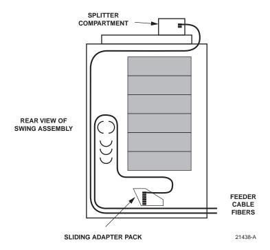
Figure 15. Feeder Cable Typical Configuration
