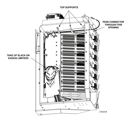
Figure 33. Re-Routing the Feeder Cable Fiber
