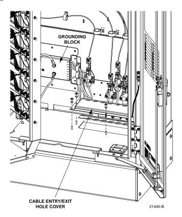
Figure 19. Cable Entry/Exit Hole Cover
