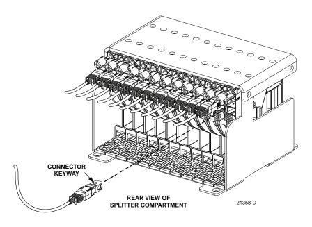
Figure 34. Feeder Cable Connector
