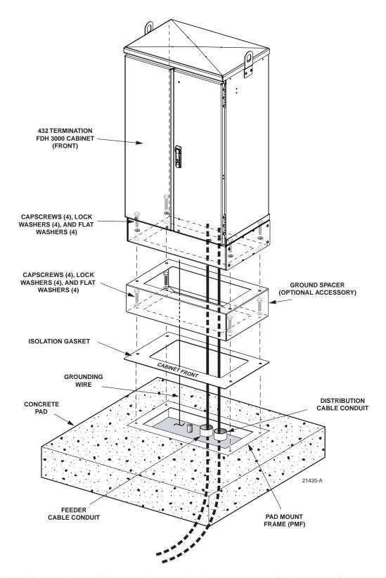
Figure 12. Mounting the 432 Termination FDH 3000 Pedestal-Mount Cabinet on the Concrete Pad
