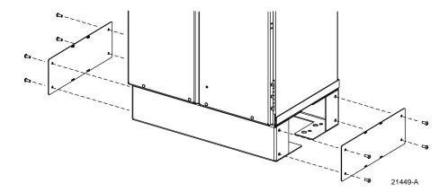
Figure 6. Removing Side Access Covers From Ground Spacer/Riser
