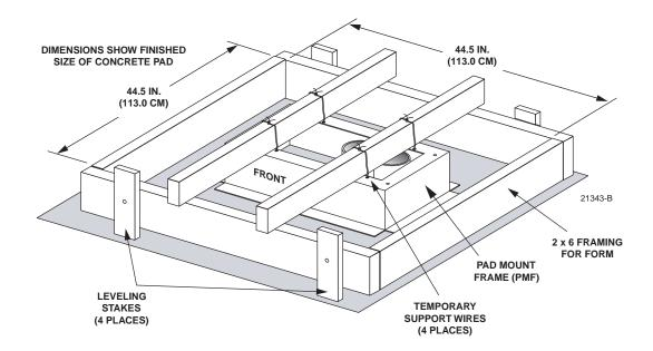
Figure 11. Concrete Pad Framing
