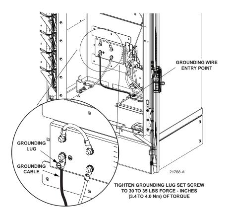
**Figure 14. Grounding Wire Connection To Cabinet**
