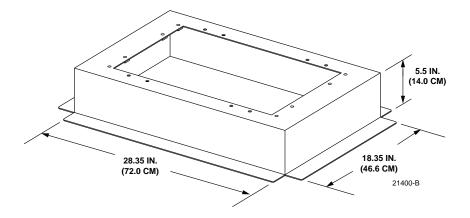
**Figure 8. Pad Mount Frame Dimensions**
