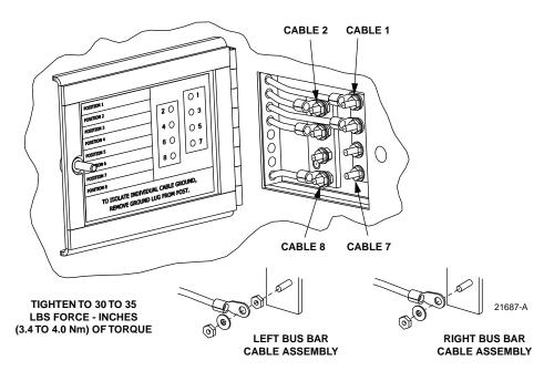
Figure 26. Cable Grounding System - Exterior View
