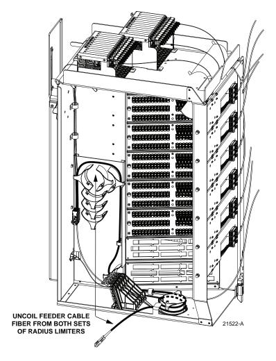
Figure 32. Uncoiling the Feeder Cable Fiber
