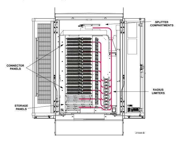
Figure 27. Routing Splitter Output Fibers
