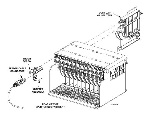
Figure 36. Splitter Compartment Adapter Replacement
