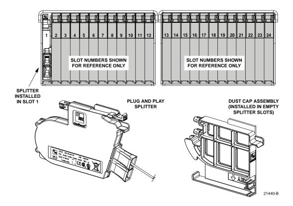
Figure 17. Splitter Module Installation
