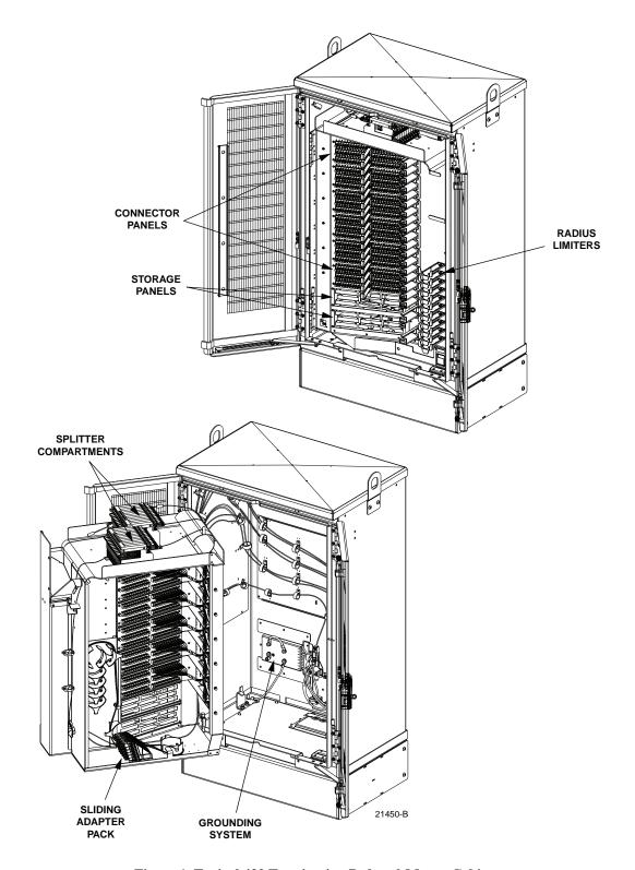
Figure 1. Typical 432 Termination Pedestal-Mount Cabinet
