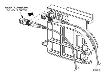
Figure 30. Installing Patch Cord Connector in Dust Cap Assembly
