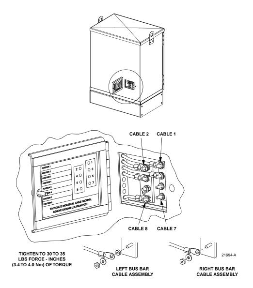
Figure 39. Grounding Block Access Cover
