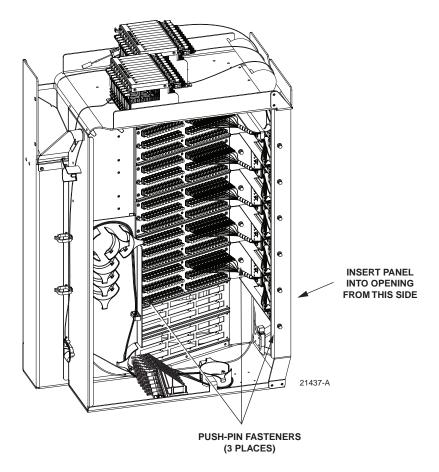
Figure 22. Placing Distribution Panel In Position For Mounting
