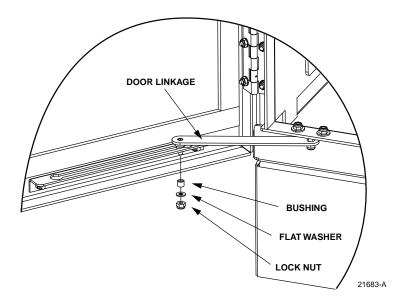
Figure 38. Door Linkage Hardware
