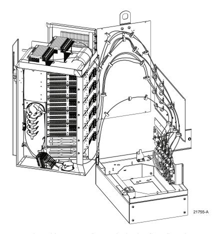
Figure 24. Route and Secure Distribution Cable Subunits
