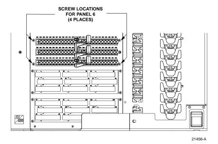
Figure 23. Secure Distribution Panel to Swing-Out Assembly
