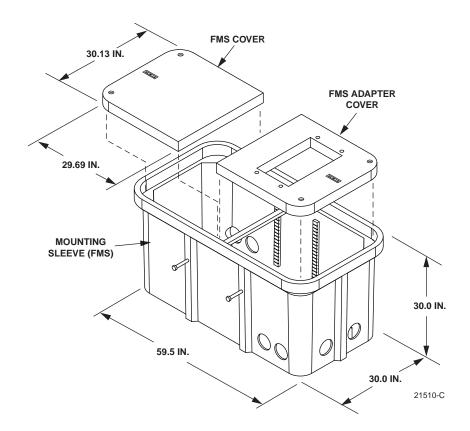
Figure 3. Mounting Sleeve (FMS-ACE100-KIT-A)
