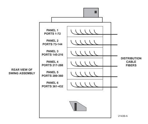
Figure 16. Distribution Cable Configuration
