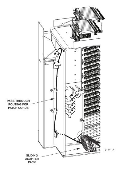
Figure 29. Routing Pass-Through Patch Cord From Sliding Adapter Pack
