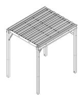
8'x12' Heavy Duty 18 gauge Protective Platform Canopy Kit (for MTC4038 platforms)
