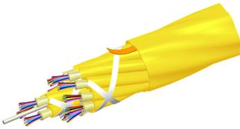
Fiber indoor cable, TeraSPEED® Low Smoke Zero Halogen Riser MPO Trunk, 144 fiber multi-unit with 12 fiber subunits, Gel-free, Singlemode G.652.D and G.657.A1, Feet jacket marking, Yellow jacket color, Dca flame rating
