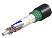
Fiber indoor/outdoor cable, TeraSPEED®, Single Jacket/Single Armor, Low Smoke Zero Halogen (LSZH), Singlemode G.652.D and G.657.A1, 36 fiber, Gel Filled, Stranded Loose Tube, Feet jacket marking, Black jacket color, Cca flame rating
