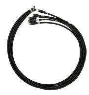
HELIAX® M-LOC Multiport cluster 4 ports SureFlex® cable assembly with Integrated Birdproofing Shell with interface type M-LOC latching male to 4.3-10 male, size 1/4", length 2 meters
