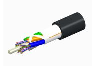
Fiber OSP cable, LightScope ZWP® Single Jacket All-Dielectric, 48 fiber, Gel-Free, Stranded Loose Tube, Singlemode G.652.D and G.657.Al, Meters jacket marking, Black jacket color
