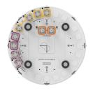
10-port small cell antenna, 4x 1695–2690, 4x 3100-4200 MHz, 2x 5150-5925 MHz, heart shape pattern, fixed tilt.
