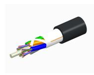
Fiber indoor/outdoor cable, TeraSPEED®, Single Jacket All-Dielectric, Low Smoke Zero Halogen (LSZH), 60 fiber, Singlemode G.652.D and G. 657.A1, Gel-Free, Stranded Loose Tube, Black jacket color, Meters cable marking, Eca flame rating
