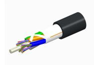
Fiber indoor/outdoor cable, TeraSPEED®, Single Jacket All-Dielectric, Low Smoke Zero Halogen (LSZH), 36 fiber, Singlemode G.652.D and G. 657.Al, Gel-Free, Stranded Loose Tube, Black jacket color, Meters cable marking, Eca flame rating
