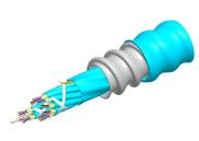
Fiber indoor cable, LazrSPEED® Riser/LSZH rated, MPO Trunk, interlocking aluminum armored, Multimode OM4, 36 fiber multi-unit with 12 fiber subunits, Gel-free, Feet jacket marking, Aqua jacket color
