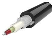
Fiber OSP cable, A2 Dual-sheathed HDPE Drop, LSZH Subunit, Loose buffer, Singlemode, G.657.A2, 1 fiber, Gel-free, Meters jacket marking, Black jacket color
