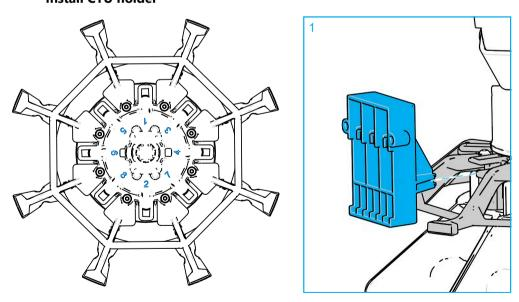
1 Select the assigned port in the starbracket and slide the two slots of the CTU holder over the flanges of that port on the star bracket.
