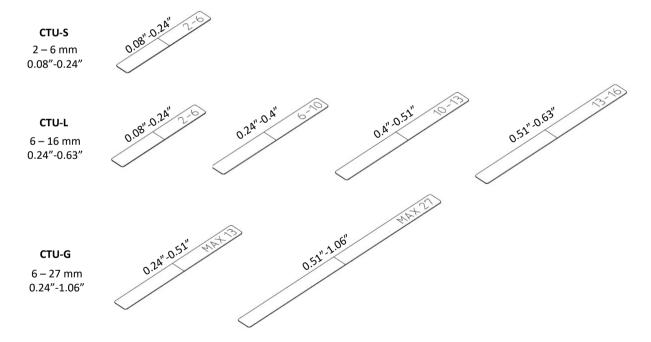
To select the correct cable retention metal strap, the diameter measured should be between the two dimensions indicated on the metal strap. For example, if the measured diameter is 15,5 mm (0.61 inch), select the 13-16 (0.51 -0.63) band.
