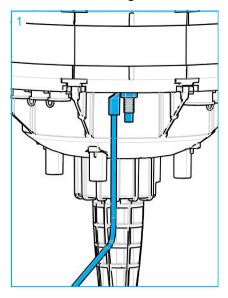
The grounding wire to connect the dummy gel seal to an object outside the closure is not included in the kit. Install this grounding wire onto the screw at the outside of the Feedthrough grounding segment, using the pre-installed star washer and nut. Tighten the nut with a hex socket wrench, size 1/2" or size 13.
