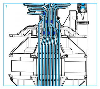
1 Bound the cable per local practice and attach the grounding wire AWG #10 to the cable. Route the grounding wire to the adjacent port using the SKG8 sealing kit.
