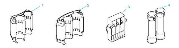
An SKG (except SKG-DUMMY and SKG-FDTHR) always contains: a CTU holder, dummy plugs and two pieces of gel seal segments (figure showing example of an SKG2 kit).
