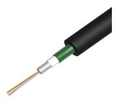
Fiber indoor/outdoor cable LSZH, Gel-filled Central Tube, CST, 4 fiber, Singlemode G.652.D and G.657.A1, Meters jacket marking, Black jacket color
