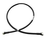
HELIAX® 1/2" Superflexible Fire retardant SureFlex® Jumper with interface types 4.3-10 Male and 4.3-10 Male, 3m, with black non-halogenated fire retardant polyolefin jacket
