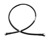
HELIAX® 1/2" Superflexible Fire retardant SureFlex® Jumper with interface types 4.3-10 Male and 4.3-10 Male, 4m, with black non-halogenated fire retardant polyolefin jacket
