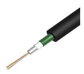
Fiber indoor/outdoor drop cable, LSZH, 2-fiber, Gel Central Tube, CST, Multimode OM3, Meters jacket marking, Black jacket color
