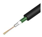
Fiber indoor/outdoor drop cable, LSZH, Gel-filled Central Tube, CST, 8 fiber, Multimode OM3, Meters jacket marking, Black jacket color
