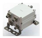
Twin Diplexer, 703-768/791-935 MHz, DC Bypass on all frequency ports, 4.3-10 connectors
