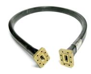
FlexTwist® Flexible Twist for WR34, 22.0–33.0 GHz, with interface types PBR260 and UBR260, 600 mm
