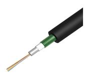
Fiber OSP cable, PE, Gel-filled Central Tube, CST, 6 fiber, Singlemode G. 657.A1, Meters jacket marking, Black jacket color
