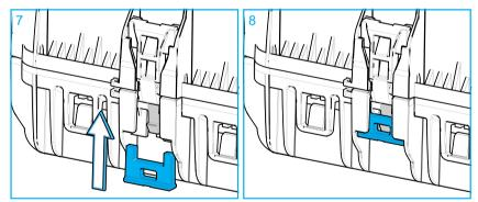
7 Re-install the lock of the hinge in the base. (For left and right position only.)8 Lock installed.
