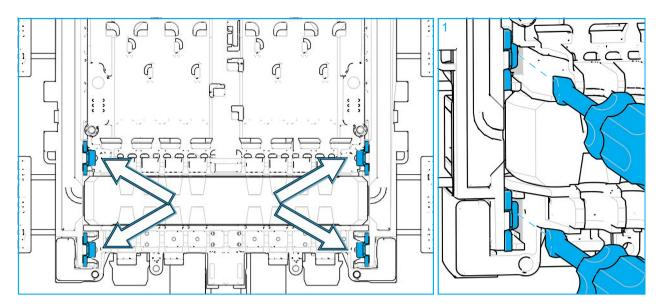
1 The 4 snap hooks at the bottom position can be released with a small screw driver.
