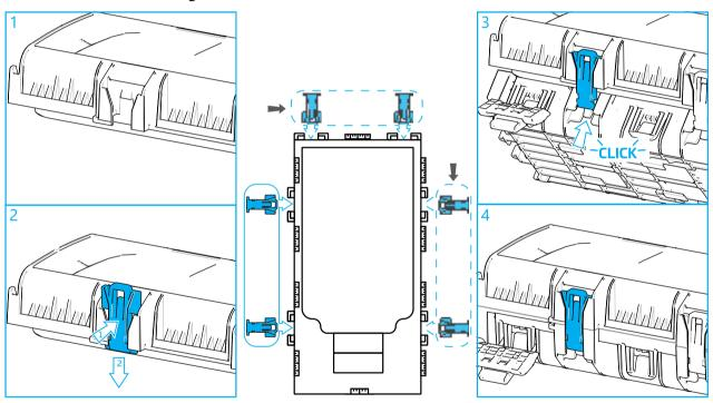
The hinges can be installed on the left, right or at the top of the cover.
