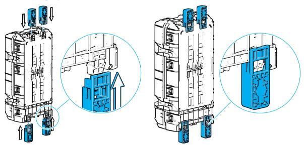
1 Mount the clips on the base on the 4 positions as shown.
