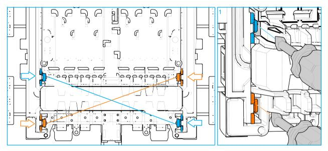
1 The 2 or 4 yellow snaps can be released with a small screw driver. If only 2 yellow snaps are installed, they are installed diagonal (either the blue positions or the orange positions).
