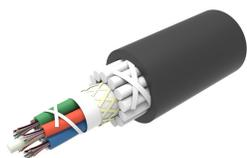
Indoor/Outdoor Low Smoke Zero Halogen, TeraSPEED® GRP Armoured, Stranded Loose Tube Fiber Optic Cable, 72-fiber, Singlemode OS2, Gel-filled, black. Provides Rodent Resistance.
