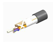
Fiber indoor/outdoor cable, LazrSPEED®, Single Jacket All-Dielectric, Plenum Rated, , 12 fiber multimode OM5, Gel-Free, Stranded Loose Tube, PVDF jacket, Black jacket color, Feet cable marking
