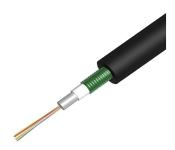
Fiber indoor/outdoor cable LSZH, Gel-filled Central Tube, CST, 2 fiber, Singlemode G.652.D and G.657.Al, Meters jacket marking, Black jacket color
