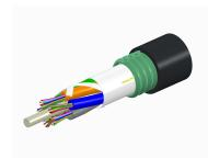
Fiber OSP cable, LightScope ZWP® Single Jacket/Single Armor, Gel-Free, 48 fibers, Stranded Loose Tube, Singlemode G.652.D and G.657.Al, Meters jacket marking, Black jacket color
