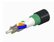
Fiber OSP cable, LightScope ZWP® Single Jacket/Single Armor, Gel-Free, 48 fibers, Stranded Loose Tube, Singlemode G.652.D and G.657.Al, Meters jacket marking, Black jacket color
