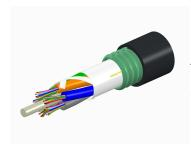
Fiber OSP cable, LightScope ZWP® Single Jacket/Single Armor, 288 fiber, Gel-Free, Stranded Loose Tube, Singlemode G.652.D and G.657.Al, Meters jacket marking, Black jacket color
