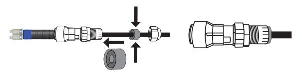
Wrap the rubber split grommet around the jacketing with the stepped end towards shroud body. Push gasket into the clamping tynes. Approximately 0.9 mm will protrude from the tynes when fully installed.
