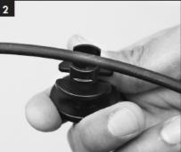
Place the open end of hanger under the cable.
