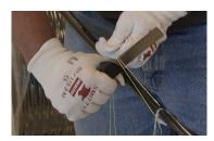
Apply Electrical Tape to Protect Breakout
