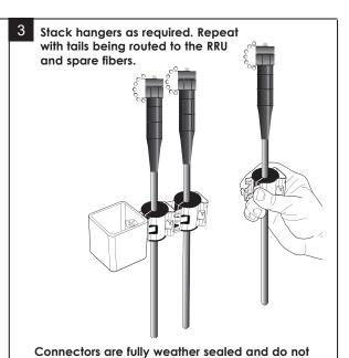
require additional weatherizing. Unused power conductors should be left with the protective cap
