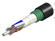
Fiber indoor/outdoor cable, loose tube gel-filled CST, 144 fiber, Singlemode G.652.D and G.657.Al, Meters jacket marking, Black jacket color
