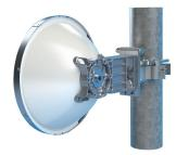
0.3 m | 1 ft ValuLine® High Performance Low Profile Antenna, single-polarized, 21.200–23.600 GHz, OEM custom flange, white antenna, polymer white radome without flash, standard pack—one-piece reflector
