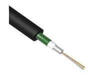
Outside Plant Fiber Optic Cable, HDPE, 12-fiber, Multimode, OM3, loose tube, gel-filled. Provides Rodent Resistance.
