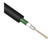
Outside Plant Fiber Optic Cable, HDPE, 12-fiber, OS2, loose tube, gel-filled. Provides Rodent Resistance.
