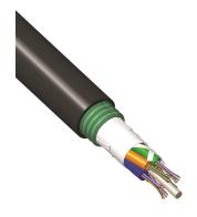
Fiber Optic Outside Plant Cable, 48-core, ECSS (Electro Chrome Coated Steel) Armored, Loose-tube, Gel-filled, 9/125 µm, OS2, Singlemode, Black cable jacket
