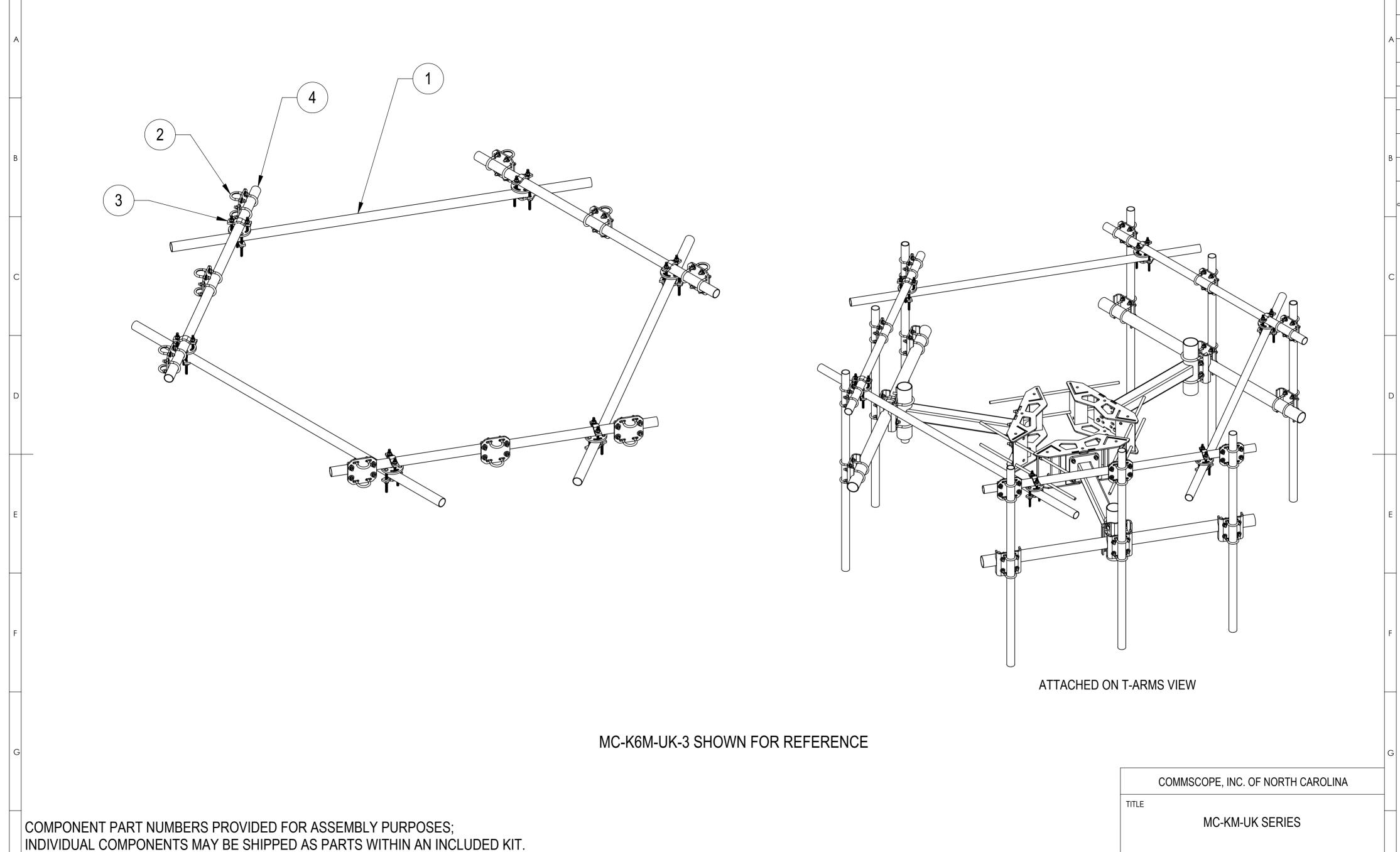
ITEM PART NO. DESCRIPTION WEIGHT NOTE MT-651-108 Ø 2.375" OD X 108" PIPE 25.93 LBS 3 PART NO. AND QTY SEE INDIVIDUAL DRAWING 2 XP-2020 7.77 LBS PART NO. AND QTY SEE INDIVIDUAL DRAWING CROSSOVER PLATE KIT, 2-3/8 OD X 2-3/8 OD 9 XP-R CROSSOVER PLATE, ROUND, UP TO 3.5" OD 3 6.20 LBS PART NO. AND QTY SEE INDIVIDUAL DRAWING Ø 2.375" OD X 84" PIPE PART NO. AND QTY SEE INDIVIDUAL DRAWING 4 MT-651-84 3 20.35 LBS
